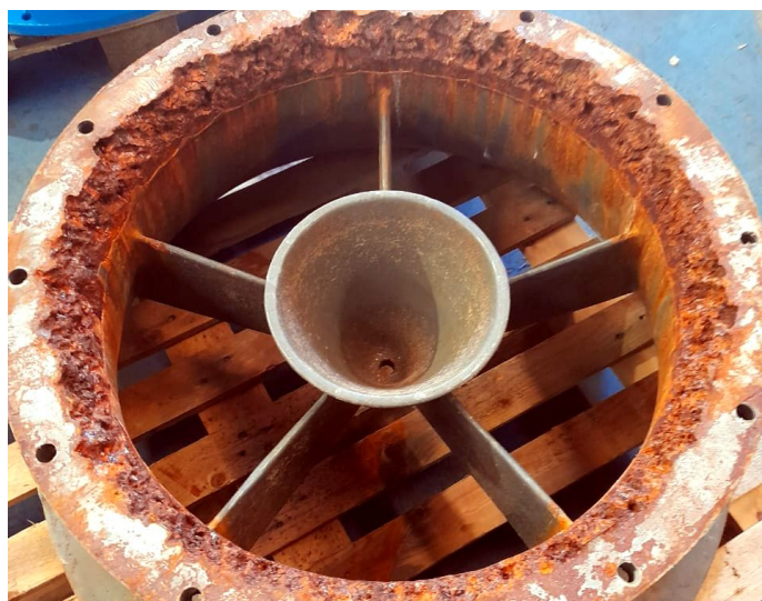
RECEIVED • CORRODED BEYOND ECONOMIC REPAIR
